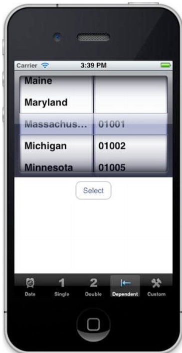
Figure 7-22. Do we really want the two components to be of equal size? Notice the clipping of a long state name.
