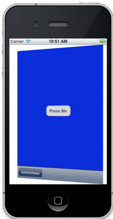
Figure 6–19. One view transitioning to another, using the flip style of animation
