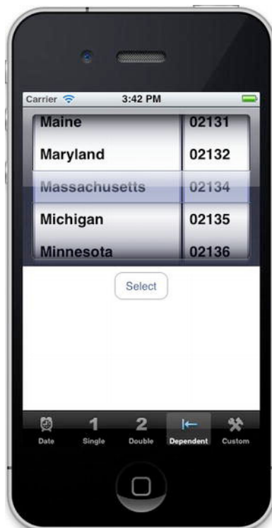
Figure 7–5. In this picker, one component is dependent on the other. As you select a state in the left component, the right component changes to a list of ZIP codes in that state.
